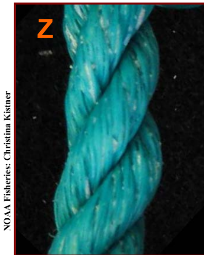
Z twist configuration of the webbing.
