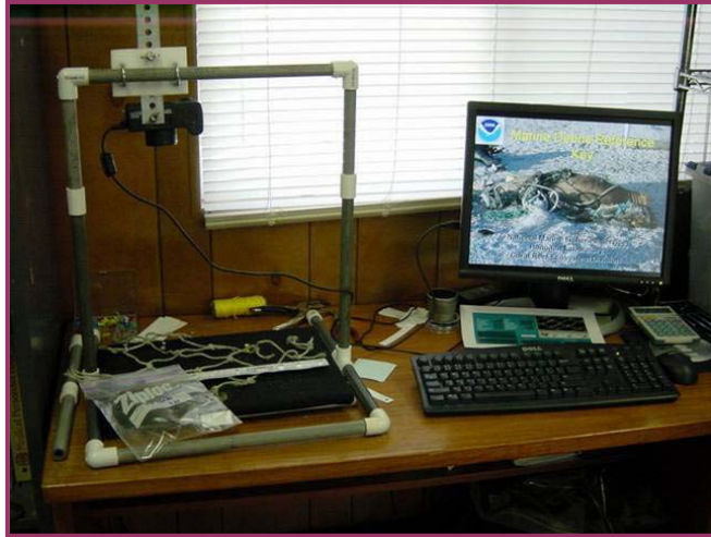
Photo mount used to capture the webbing images represented in the Ghost Net Identification Database.
