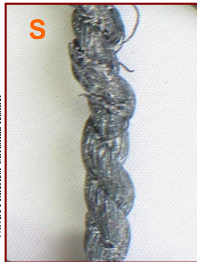
S twist configuration of the webbing.
