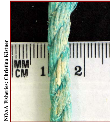
Twine diameter measured in millimeters.
